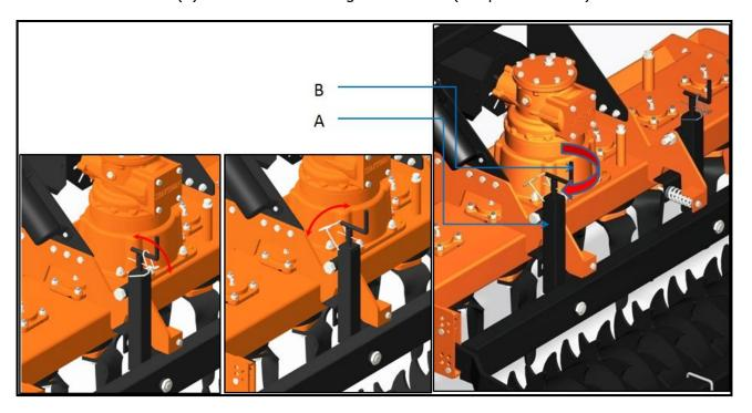
It is recommended to set the bar position at 4-5 cm higher compared to the position of the roller on the ground.
