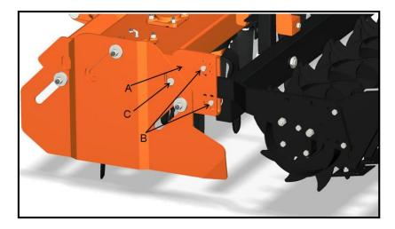
Operator can adjust the roller height in eight different positions, by inserting the two adjusting pins (B) into the holes immediately above and below the roller's swinging arms, according to the desired working height.
