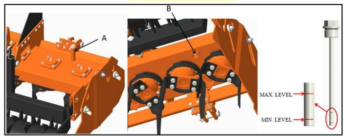
If the mark is below the minimum, fill up oil till the correct level is restored.
