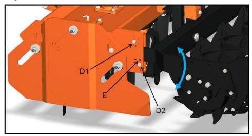
This configuration can be useful in case the machine meet an obstacle during operation, allowing the machine to overcome it without damaging the roller, thanks to the swinging arms, and obtaining a nearly uniform leveling of the ground.
