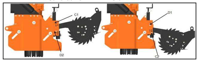
The roller can be left in floating configuration, free to follow the ground contour, by positioning the adjusting pin (D2) in a hole lower to position (E) immediately below to the connecting arm, or by removing it altogether.
