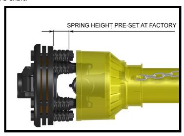
An adjustment can be done, however, when the clutch slipping is too frequent, which means that the calibration is too low. In this case, the tightening of nuts over the compressed springs will give an increase in torque transmissible. On the contrary, a loosening of the nuts over the springs will give a decrease in torque transmissible.
