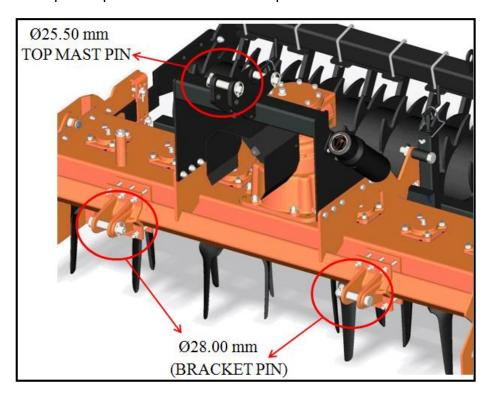
If the dimension of the pins is not corresponding to Category 2, contact the Manufacturer or the Dealer to obtain the pins of right dimension.
