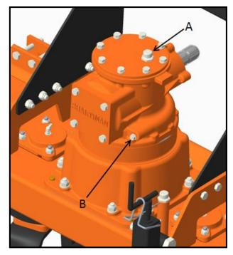
If the mark is below the minimum, fill up oil till the correct level is restored.
